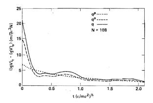
FIG. 1. Heat flux autocorrelation functions of q,  $q^0$ , and  $q^p$ for N = 108 and  $T = 0.546\epsilon/k_B$ . Only the initial portions of the correlation functions are shown.
