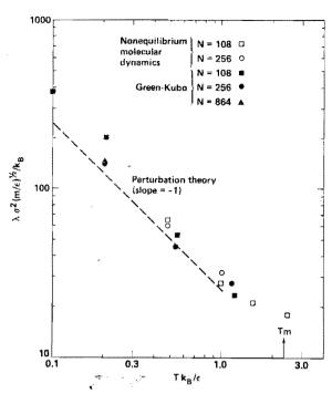
FIG. 3. Thermal conductivity from equilibrium Green-Kubo, nonequilibrium molecular dynamics, and phonon perturbation theory. The melting temperature is indicated by the vertical arrow labeled  $T_m$ .
