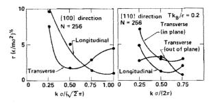
FIG. 4. Phonon lifetimes as a function of k in the [100] and [110] directions, for N=256 and  $T=0.2\epsilon/k_B$ . The solid lines are drawn as a visual aid to identify the various branches. In the [110] direction the two transverse modes are not degenerate and have different frequencies for motion in the plane of the k vector and perpendicular to this plane.
