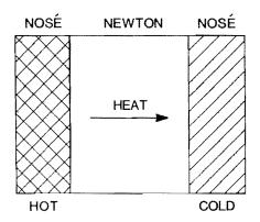
FIG. 1. Schematic of a boundary-bulk-boundary (Nosé-Newton) nonequilibrium system. Here, atoms in the left-most boundary region are Nosé thermostatted at a high temperature; atoms in the middle (bulk) region are governed by Newton's equations; atoms in the right-most boundary region are Nosé thermostatted at a low temperature. Heat flows through the bulk region from left to right. (Vertical walls separate particles in the three regions via elastic, specular collisions.)
