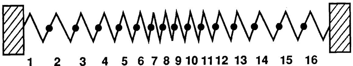
Figure 2. 16-spring anharmonic oscillator chain studied by Fermi, Pasta, Ulam, Tuck, and Menzel at Los Alamos. The typical starting condition was the lowest-frequency "mode" shown in the Figure, with quadratic or cubic forces added to the Hooke's-Law linear forces.
