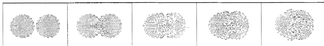
FIGURE 3. Snapshots of the low-speed inelastic cold-welding of two embedded-atom particles.
