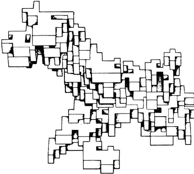
Fig. 8. Perspective view of a damaged region in a computer simulation of radiation damage in  $\alpha$ -iron. The initial energy responsible for the damage was 5 keV. From work by J. R. Beeler, Jr., cited by Vineyard (1972).
