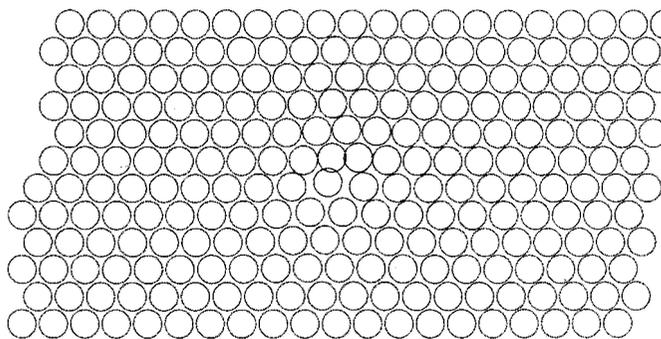
FIG. 1. Geometry for studying the structure of edge dislocations using molecular dynamics and elasticity theory. The particles along the upper and lower edges of the strip are clamped so that the stress well ahead (right) of the dislocation is pure shear and that far behind (left) the dislocation is zero.
