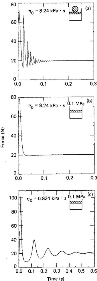
Fig. 2. Force-time history on the confining piston. (a) Calculation includes bouncing of the weight on the piston. (b) and (c) Weight-piston interaction replaced by an average downward pressure of 0.1 MPa.
