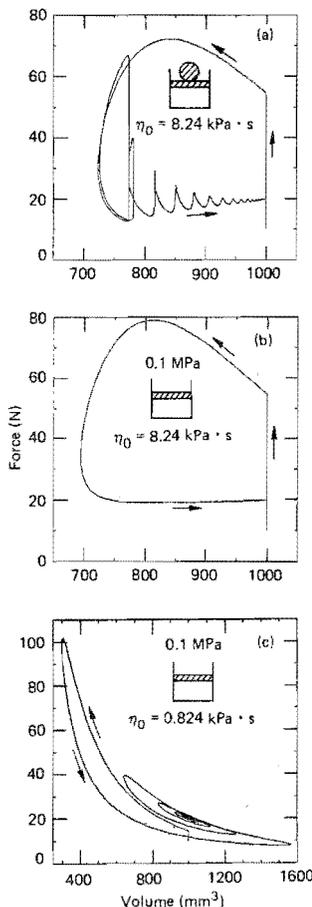
Fig. 5. Force on the piston versus volume of the gas. The area under each curve is  $-mghA$ . (a) Calculation includes bouncing of the weight on the piston. (b) and (c) Weight-piston interactions replaced by an average downward pressure of 0.1 MPa.
