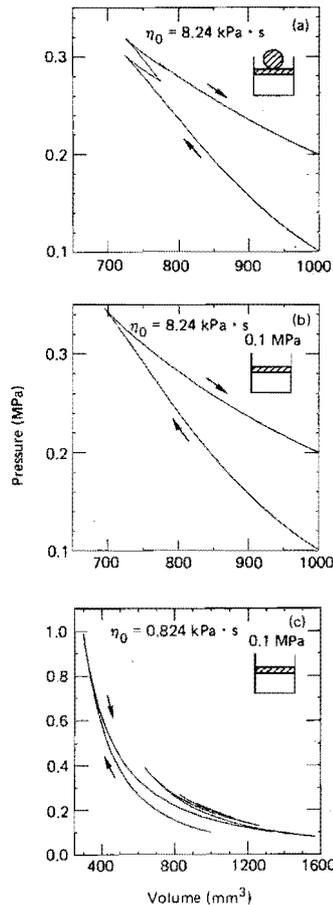
Fig. 6. Pressure-volume diagram. (a) Calculation includes bouncing of the weight on the piston. (b) and (c) Weight-piston interactions replaced by an average downward pressure of 0.1 MPa.
