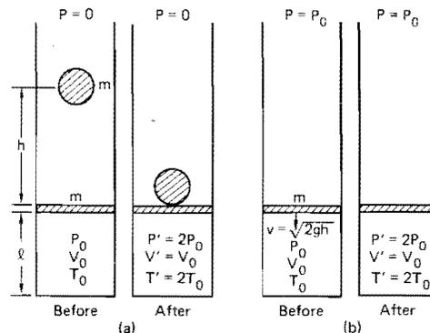
Fig. 1. Schematic diagram for problem I. (a) Exact treatment includes elastic bouncing of the weight on the piston. (b) Weight-piston interactions replaced by an averaged downward pressure  $P_0$ .
