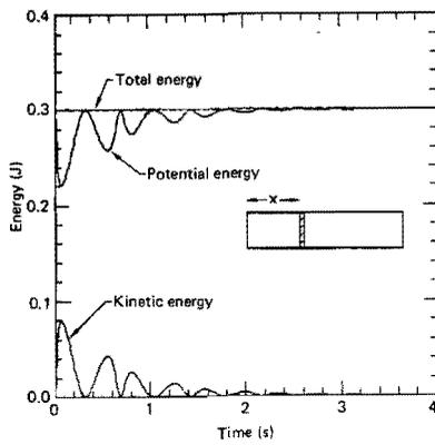
Fig. 10. Energy partition as a function of time.  $m = 0.1$  kg,  $\eta_0 = 0.2$  kPa sec,  $\alpha = 0.8$ .
