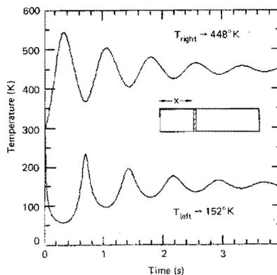
Fig. 9. Temperature of the gas on both sides of the piston as a function of time.  $m = 0.1$  kg,  $\eta_0 = 0.2$  kPa sec,  $\alpha = 0.8$ .
