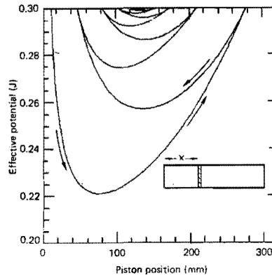
Fig. 12. Effective potential for piston motion.
