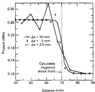
Fig. 15. Pressure profile within the shock front.
