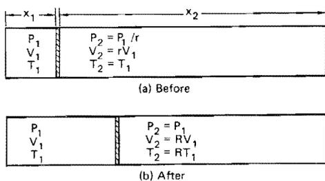
Fig. 7. Schematic diagram for problem II. Solutions for the case  $r = 50$  are illustrated in Figs. 8-13.
