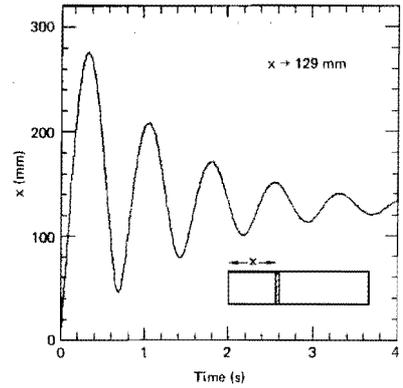
Fig. 8. Piston position as a function of time.  $m = 0.1$  kg,  $\eta_0 = 0.2$  kPa sec,  $\alpha = 0.8$ .
