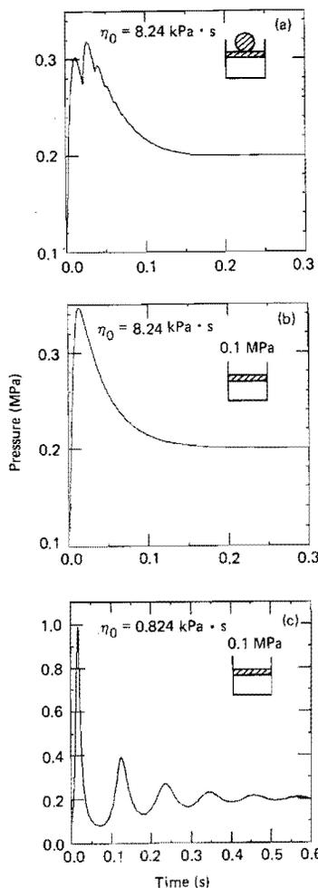
Fig. 3. Time variation of the mean pressure  $NkT/V$  in the gas. (a) Calculation includes bouncing of the weight on the piston. (b) and (c) Weight-piston interactions replaced by an average downward pressure of 0.1 MPa.
