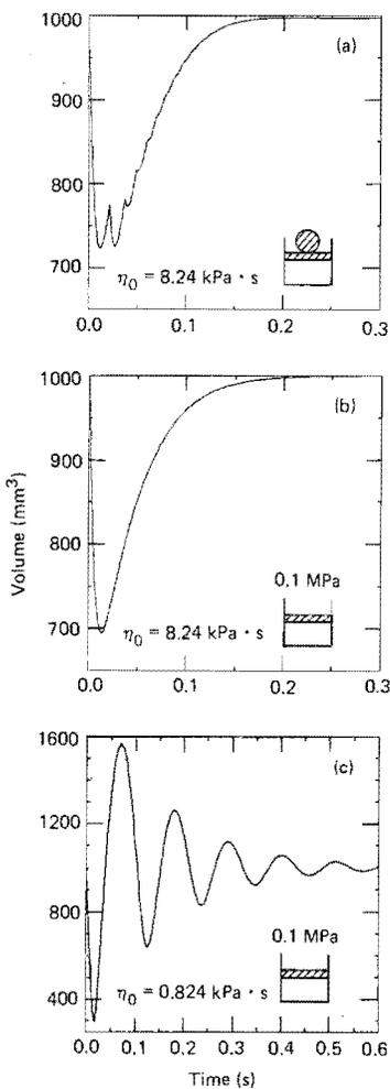
Fig. 4. Volume-time history. (a) Calculation includes bouncing of the weight on the piston. (b) and (c) Weight-piston interactions replaced by an average downward pressure of 0.1 MPa.
