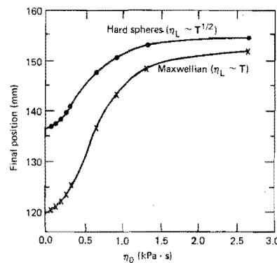
Fig. 13. Dependence of the final position on the transport properties.
