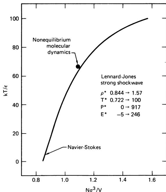
FIG. 5. Density-temperature states traversed in the shock wave according to continuum mechanics are shown as a full curve. The  $\bullet$  indicates the state at the shock-wave center according to 4800-particle nonequilibrium molecular dynamics.
