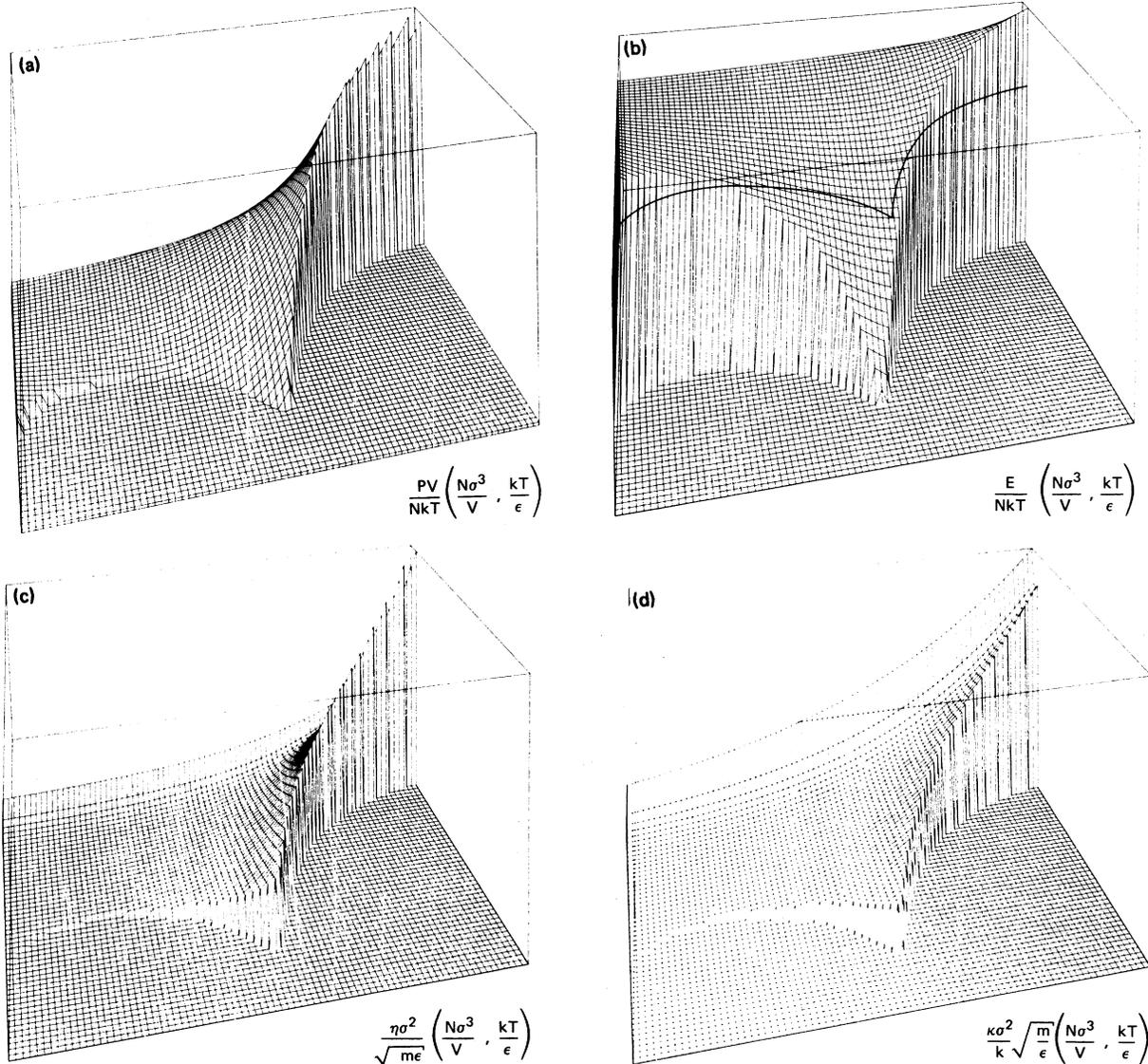
FIG. 4. Pressure, energy, shear viscosity, and thermal conductivity for the Lennard-Jones potential. The independent variables,  $\exp(-\epsilon/kT)$  and  $N\sigma^3/V$  span a temperature range  $0 < kT/\epsilon < 100$  and a reduced density range  $0 < N\sigma^3/V < 1.60$ . The dependent variables span the ranges  $0 < PV/NkT < 16$ ,  $-8 < ENkT < 3.5$ ,  $0 < \eta\sigma^2(m\epsilon)^{-1/2} < 50$ , and  $0 < \kappa\sigma^2(m/\epsilon)^{1/2}/k < 60$ .
