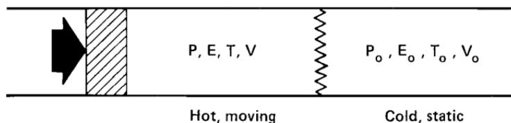
Figure 5. Steady Shockwave Generated by a Piston Compressing a Fluid
