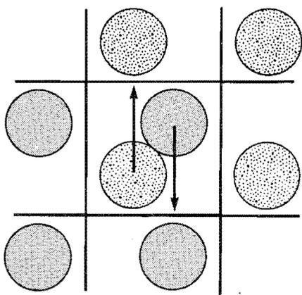
FIG. 1. Initial condition for the two-body problem discussed in the text. Periodic boundaries are used with a box length equal to twice the range of the interparticle forces.
