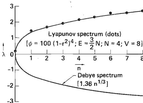
FIG. 2. Sample Lyapunov spectrum ( $3N - 3 = 9$  exponents indicated by points) for a four-particle fluid compared with the Debye spectrum (full curve). Data taken from Table II at time 10. The negative exponents match the positive exponents in absolute value for Hamiltonian systems, such as those studied here.
