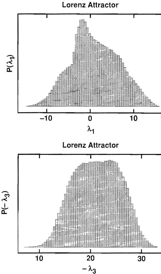
Fig. 2. Probability density for  $\lambda_1$  and for  $\lambda_3$  taken from the forward and backward versions of the attractor segment shown in fig. 1. The moments of the  $\lambda_1$  distribution constitute the usual "spectrum of multifractality".
