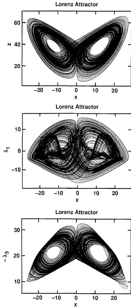
Fig. 1. Lorenz attractor trajectory corresponding to a time interval from 50 to 250 taken from a 300000-step run with timestep  $dt=0.001$  with the parameters listed in eq. (4) and initial point (11, 16, 28). The Lorenz variable  $z$  as well as the Lyapunov exponents  $\lambda_1$  and  $\lambda_3$  are plotted as functions of the Lorenz variable  $x$ .
