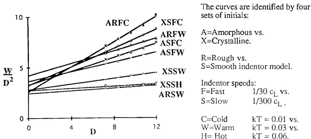
Figure 7. Variation of the reduced work of indentation,  $W_{\text{total}}/D^2$  as a function of  $D$ . The intercept gives an estimate of the combined elastic and surface energies while the slope is the plastic yield strength. The energy and length scales are given in Stillinger-Weber units<sup>4</sup> (50kcal/mole and 0.21 nm).
