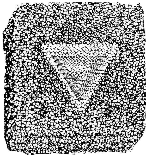
Figure 1. Top view of the indentation geometry for 32,768 particles. This is at the end of the deformation with the indenter removed.
