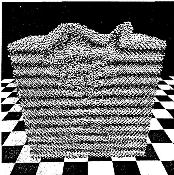
Figure 6. A cut-away view at the end of the indentation showing the plastic structure of the crystal in the region of the indentation.
