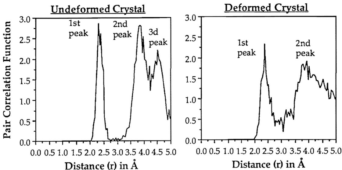
Figure 5. Pair correlation function in the volume in the upper left pattern of Figure 4a and 4b.
