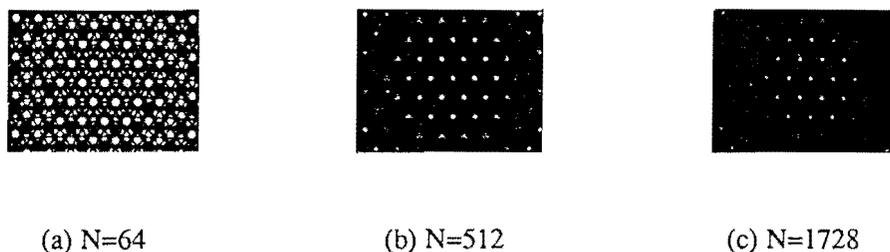
Figure 2. Size dependence of diamond-structure diffraction patterns, where  $N$  is the total number of atoms.
