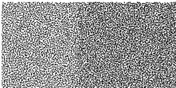
FIG. 1. Snapshot of the 12 960-particle shock wave simulation described in the text. Particles enter at the left and leave at the right. Fourth-order Runge-Kutta integration of the motion equations with a timestep of 0.025 is used.
