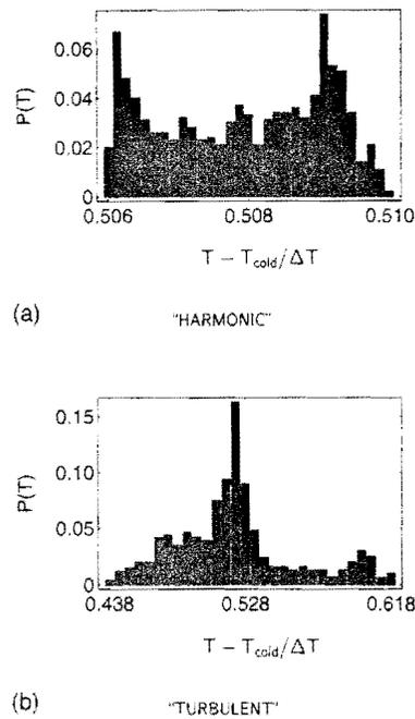
FIG. 2. The temperature-fluctuation histogram for a point at the center of the simulated cell for the (a) "harmonic" and (b) "chaotic" flows.
