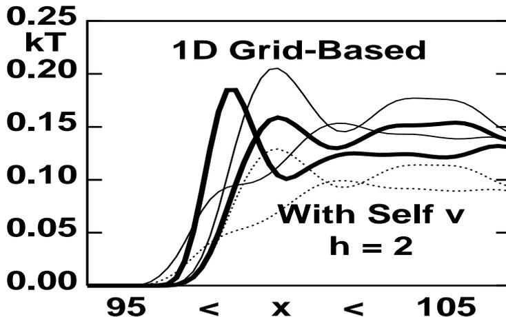
Figure 8: Temperature profiles with the same data as in Figure 7, but with a reduced averaging range,  $h = 2$ . Again, the temperatures including “self” contributions to the local velocity are shown as dashed lines. Notice the sensitivity of the maximum in  $T_{xx}^K$  to the range  $h$ . Far to the right, the “correct” hot temperature, at equilibrium, away from the shock, is  $kT = 0.13$ , based on separate equilibrium molecular dynamics simulations.
