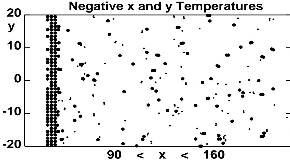
Figure 6: Particles with *negative* configurational temperatures are shown here, using the data underlying Figs. 4 and 5. The material to the right of the shock is “hot”, with cold material entering at the left. The smaller dots correspond to negative values of  $T_{xx}^\Phi$  and the larger ones to negative  $T_{yy}^\Phi$ .
