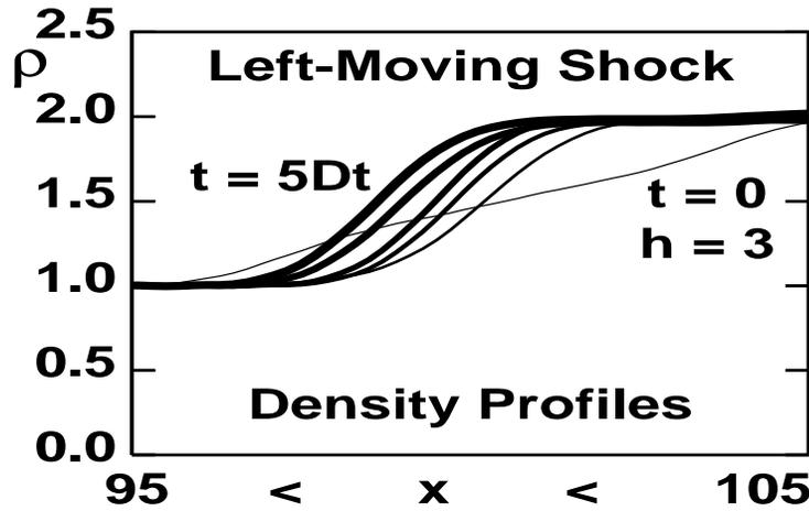
Figure 4: Density profiles at the same times as those illustrated in Figure 3. These one-dimensional density profiles were computed with Lucy's one-dimensional smooth-particle weight function using  $h = 3$  and the particle coordinates shown in Figure 3. Increasing time corresponds to increasing line thickness as the shockwave moves slowly to the left.
