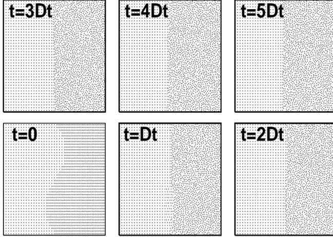
Figure 3: Particle positions in the initial condition correspond to  $t = 0$ . Those to the left of the sinewave boundary move to the right at speed  $u_s = 1.75$  while those to the right travel at speed  $u_s - u_p = u_s/2$ . Particle positions at five later equally-spaced times are shown too. The time interval  $Dt = 40/u_s$  is 2000 timesteps. The  $40 \times 40$  windows shown here would contain 1600 cold particles or 3200 hot particles at the cold and hot densities of 1.0 and 2.0.
