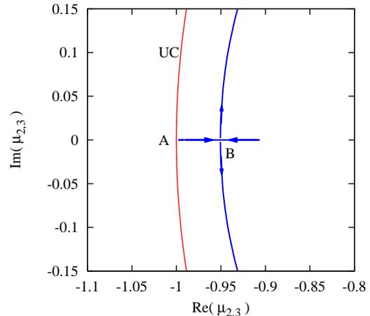
FIG. 2: (Color online) Floquet multipliers  $\mu_2$  and  $\mu_3$  in the complex plain for  $\varepsilon \geq 0.26312$ . UC denotes the unit circle, and A is the bifurcation point. The multipliers are complex conjugate to each other for  $\varepsilon > 0.26319$  as indicated by B.
