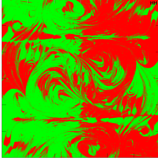
Figure 1: The sign of the local (time-dependent) value of the largest Lyapunov exponent for the Hoover-Holian oscillator is shown in the (q, p, 0, 0) plane. Because a mirror reflection of the dynamics ( perpendicular to the q axis ) changes the signs of both q and p the Figure reveals an inversion symmetry. In the upper half plane red indicates a positive exponent and green a negative. The colors are reversed in the lower half plane. The probability density in the cross-sectional plane is a simple Gaussian in q and p . Nevertheless the local Lyapunov exponents vary in a multifractal manner throughout the four-dimensional space, reflecting their sensitivity to bifurcations in their past histories. In Figures 1-4 both q and p range from -3 to +3 .
